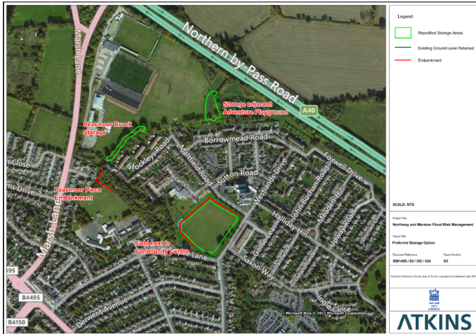
Figure 3: Outline of final scheme proposal including temporary flood storage at Northway Community Field and Court Place Farm (green outline) and natural embankments at Peasmoor Place and Northway Community Field.
